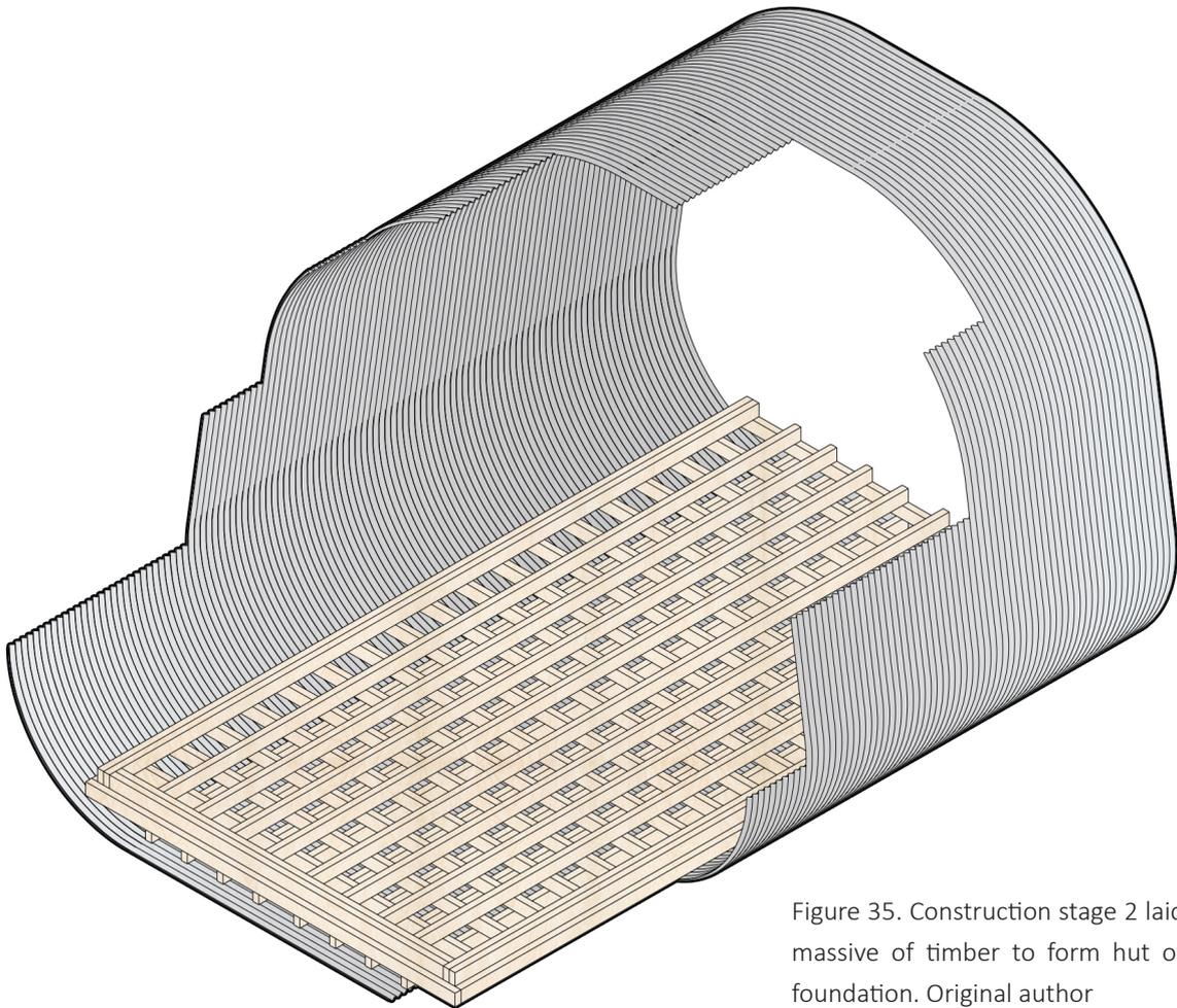
Figure 35. Construction stage 2 laid massive of timber to form hut of foundation. Original author
