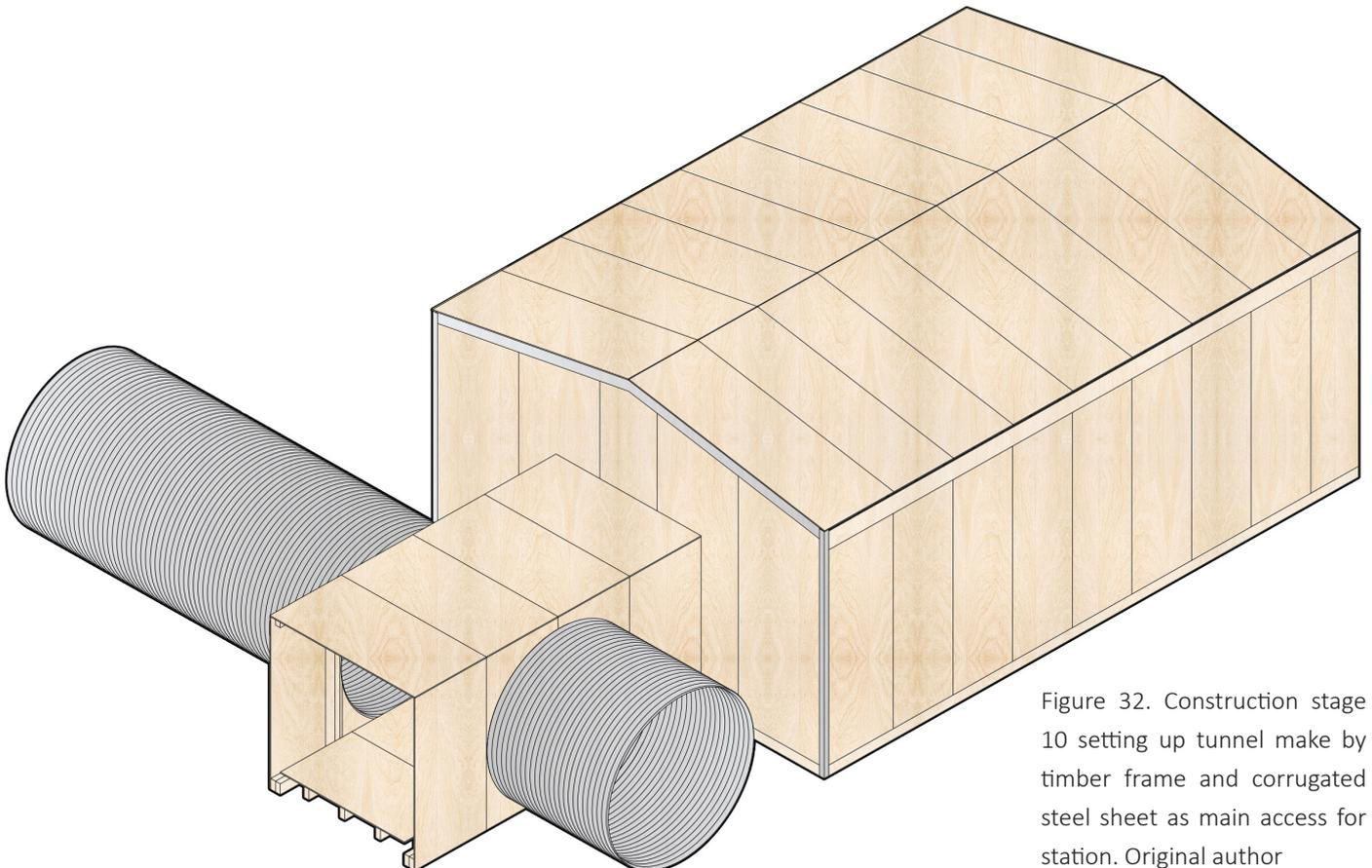
Figure 32. Construction stage 10 setting up tunnel make by timber frame and corrugated steel sheet as main access for station. Original author
