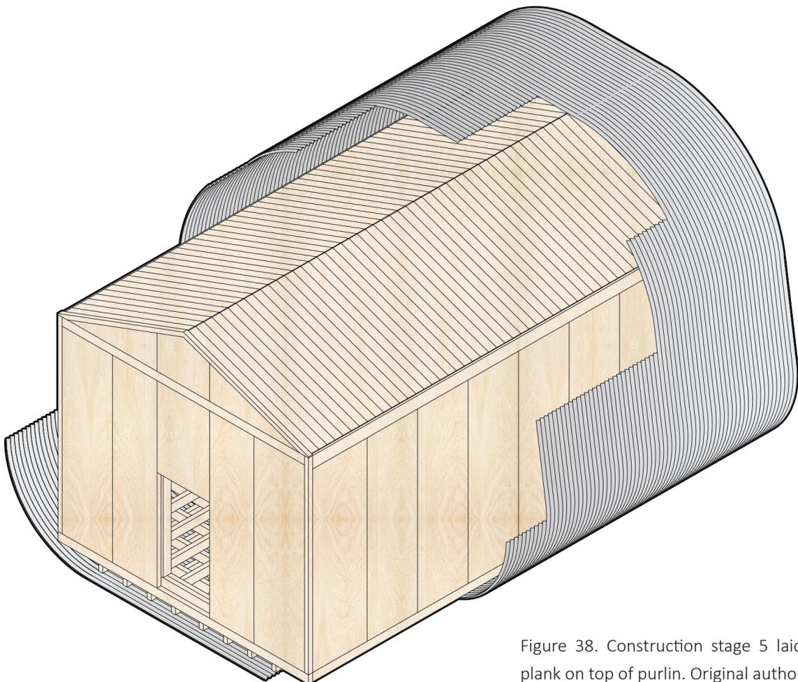
Figure 38. Construction stage 5 laid plank on top of purlin. Original author
