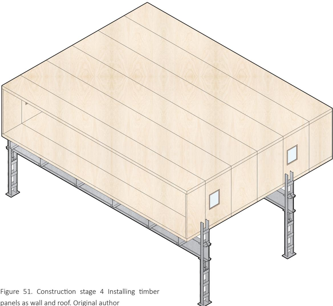
Figure 51. Construction stage 4 Installing timber panels as wall and roof. Original author
