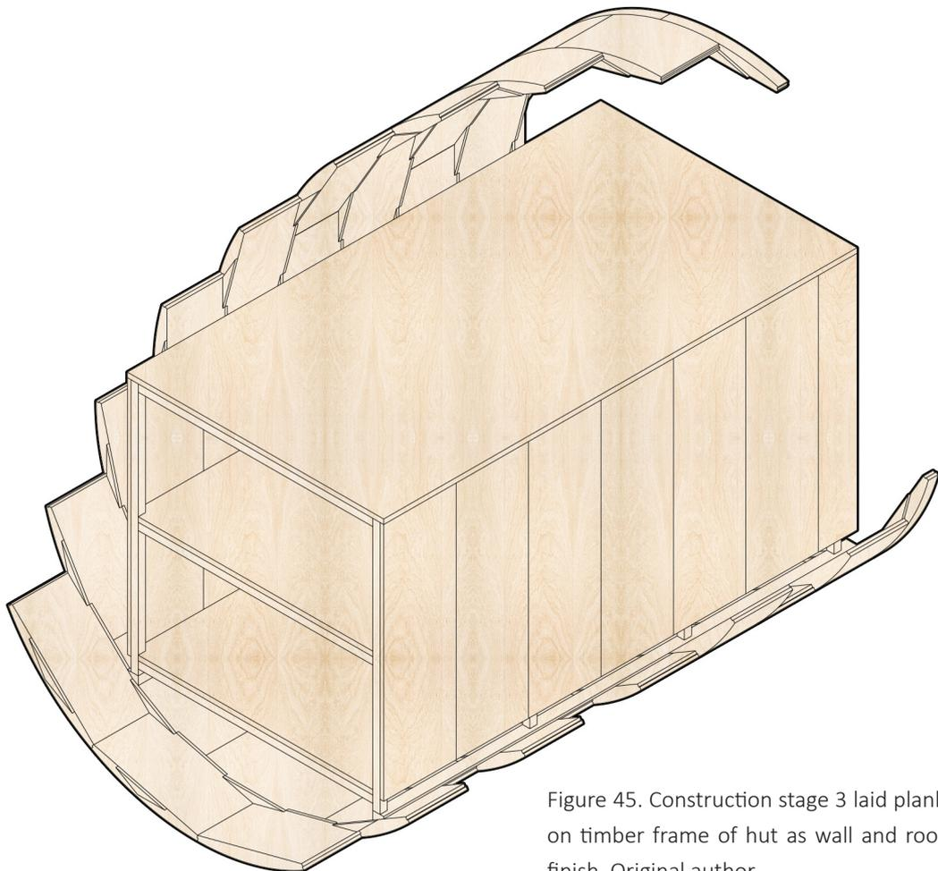
Figure 45. Construction stage 3 laid plank on timber frame of hut as wall and roof finish. Original author
