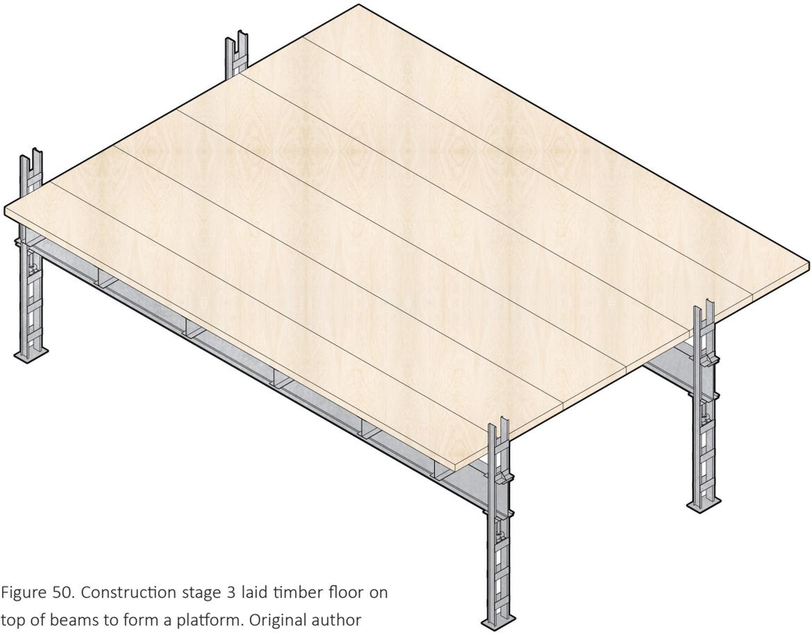
Figure 50. Construction stage 3 laid timber floor on top of beams to form a platform. Original author
