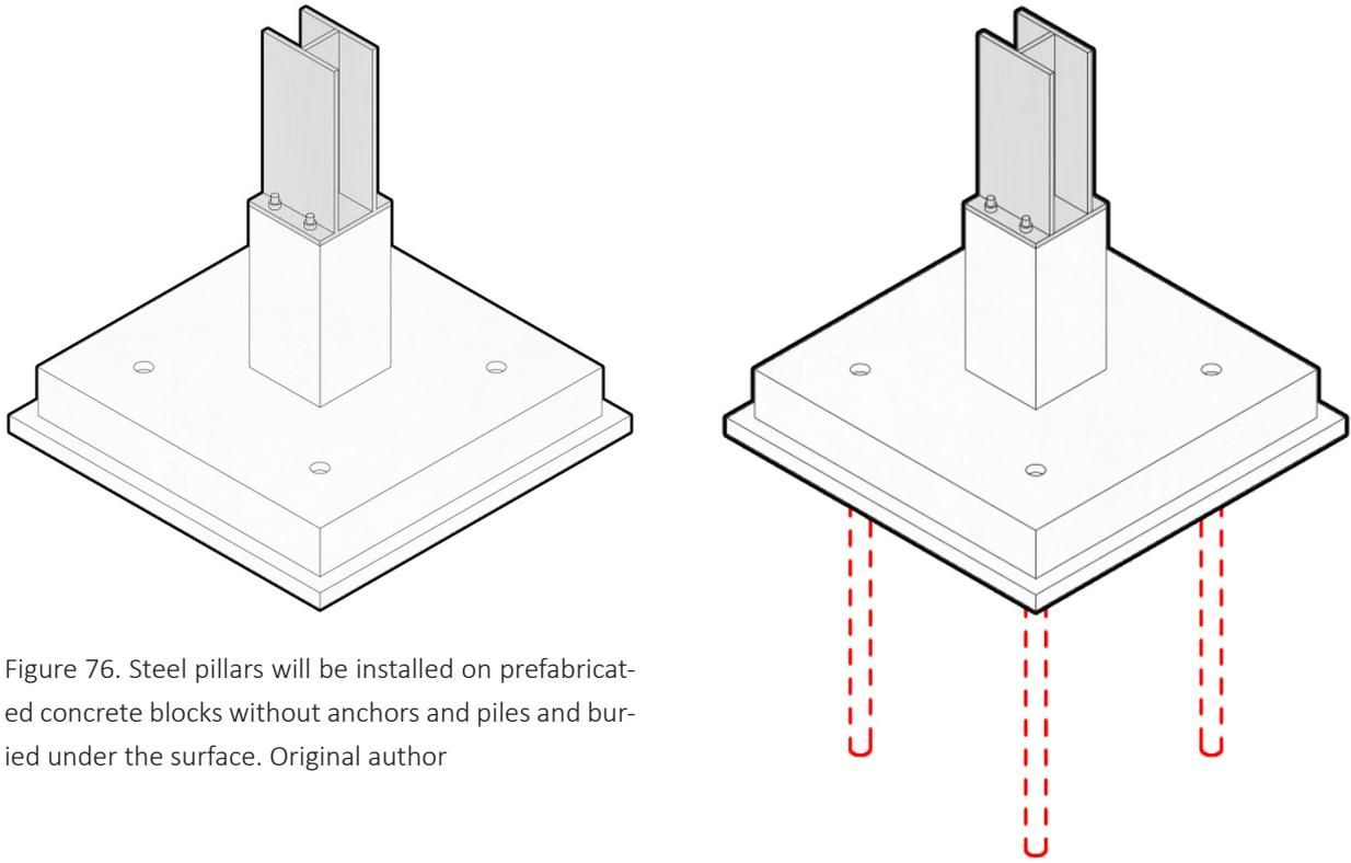
Figure 76. Steel pillars will be installed on prefabricated concrete blocks without anchors and piles and buried under the surface. Original author
