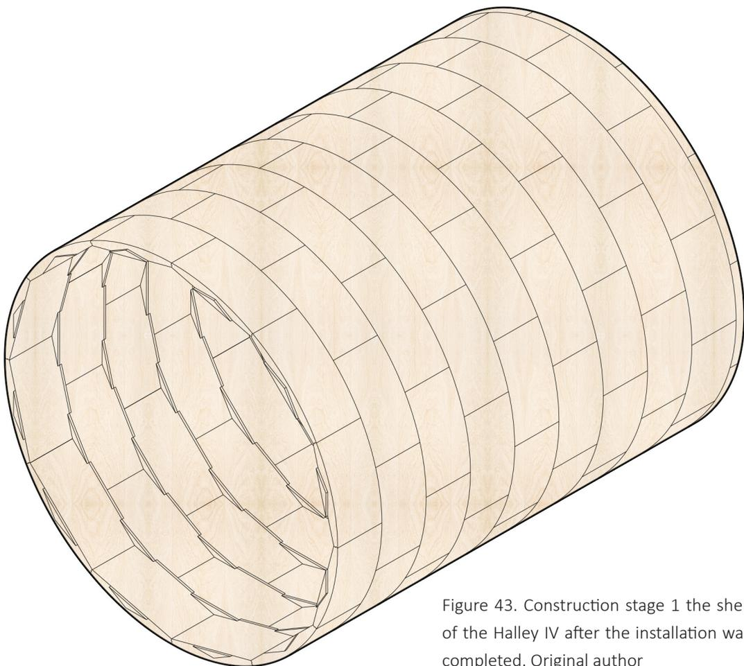
Figure 43. Construction stage 1 the shell of the Halley IV after the installation was completed. Original author
