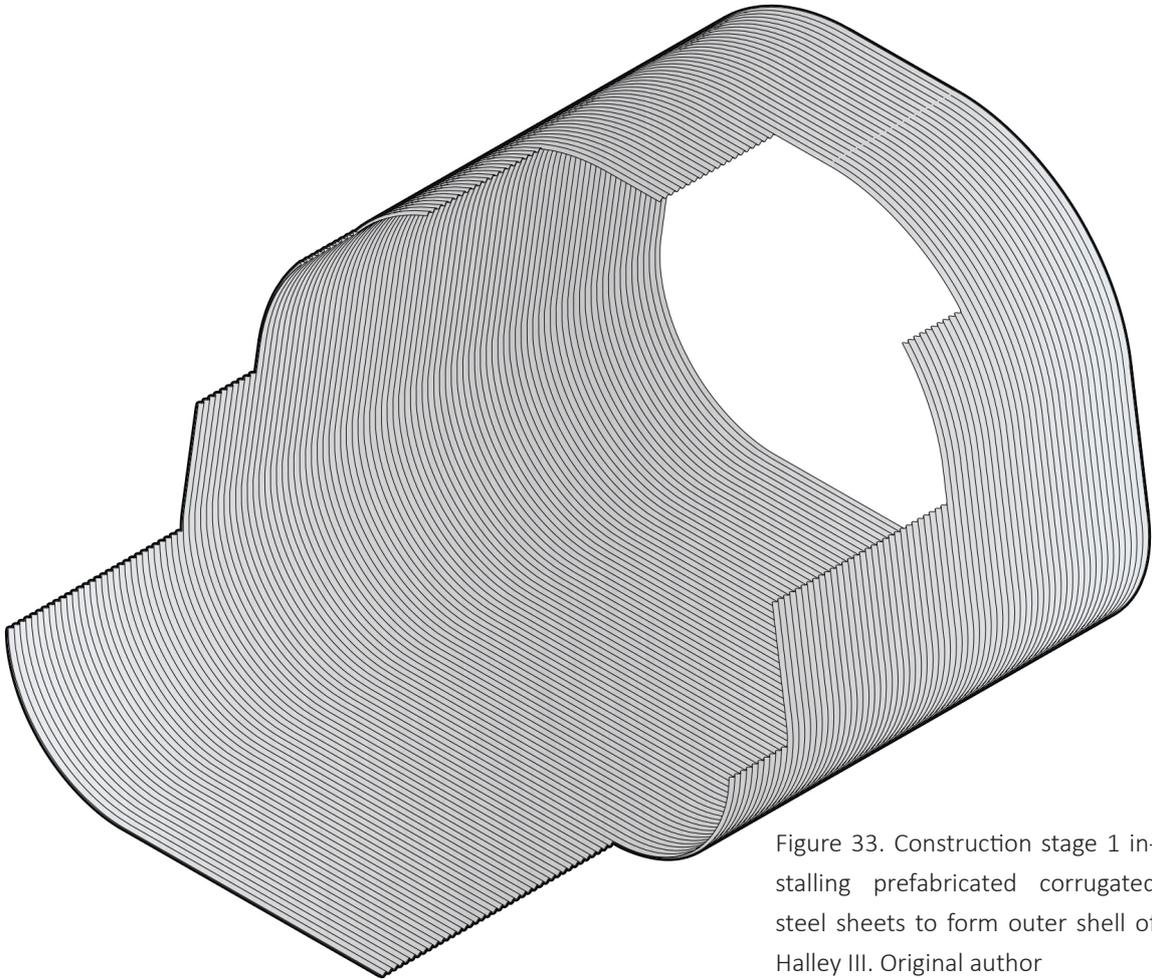
Figure 33. Construction stage 1 installing prefabricated corrugated steel sheets to form outer shell of Halley III. Original author
