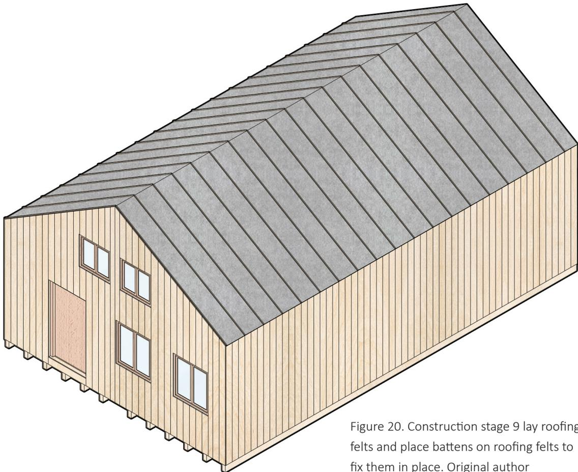
Figure 20. Construction stage 9 lay roofing felts and place battens on roofing felts to fix them in place. Original author
