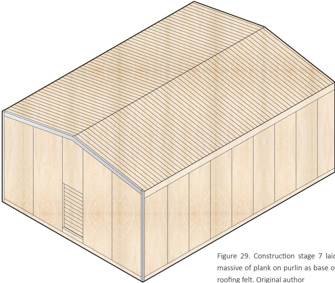
Figure 29. Construction stage 7 laid massive of plank on purlin as base of roofing felt. Original author
