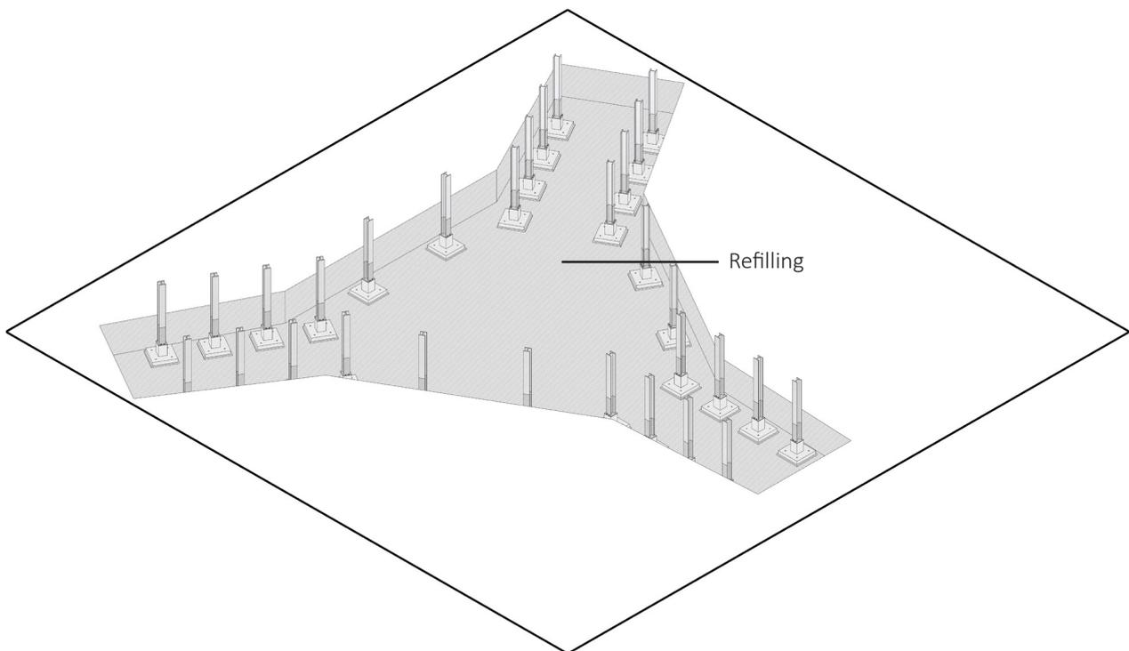
Figure 75. Foundation layout. Shallow foundation is applied to the station. Original author
