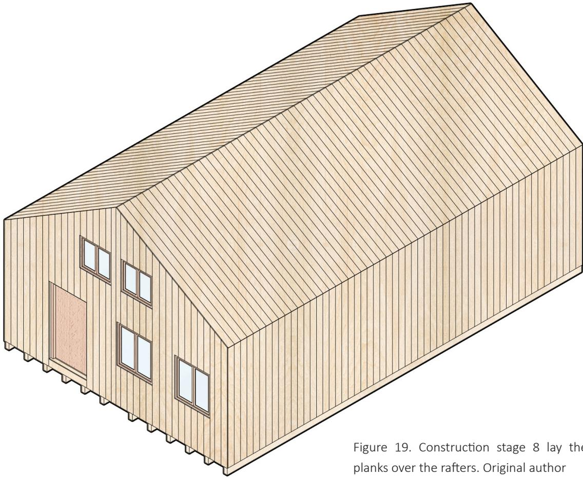
Figure 19. Construction stage 8 lay the planks over the rafters. Original author
