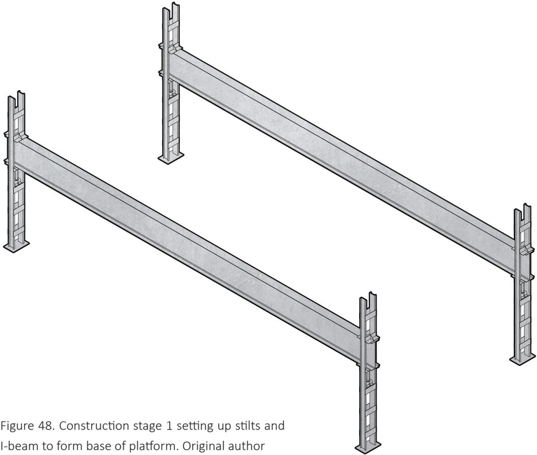
Figure 48. Construction stage 1 setting up stilts and I-beam to form base of platform. Original author
