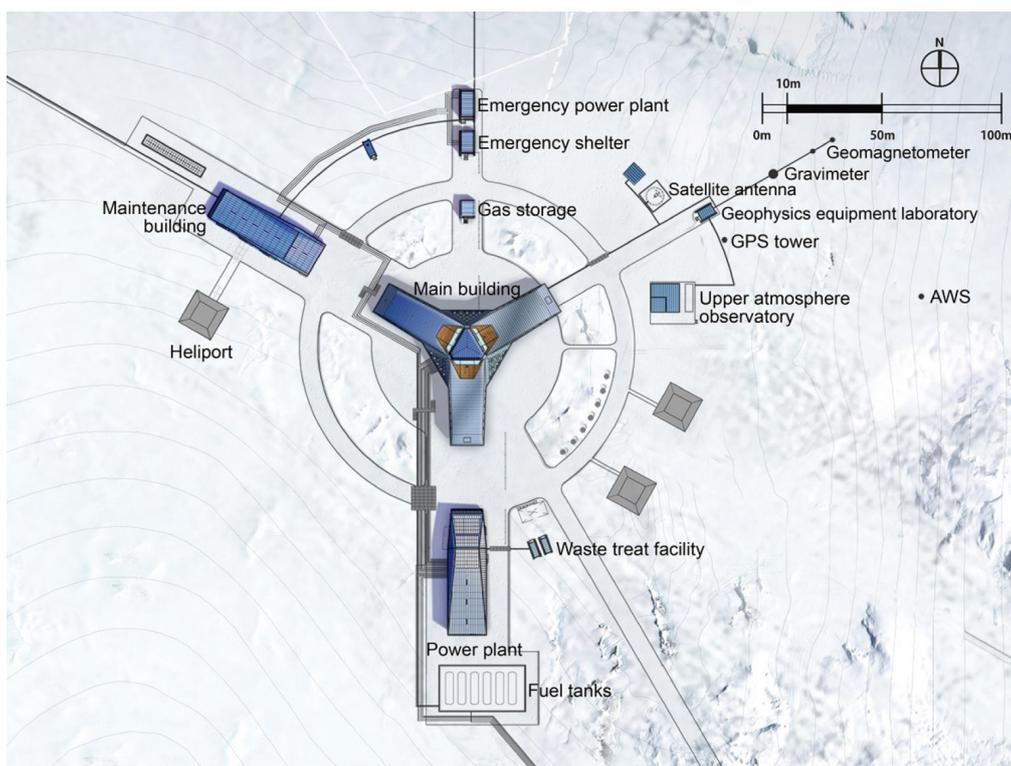
Figure 73. Layout of the Jang Bogo Station. Photo attributed to Korea Polar Research Institute & Korea Environment Institute. Source: Final comprehensive environmental evaluation, construction and operation of Jang Bogo Antarctic Research Station, Terra Nova Bay, Antarctica
