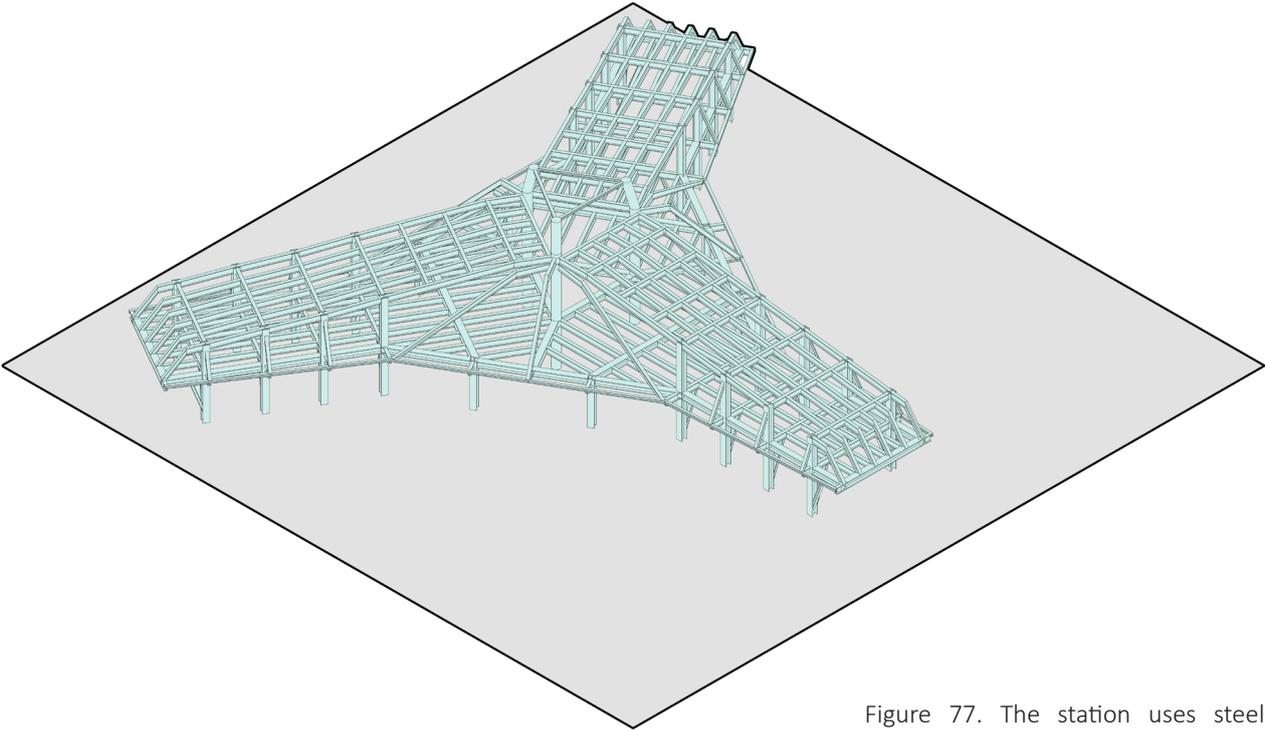
Figure 77. The station uses steel frame as structure of superstructure. Original author
