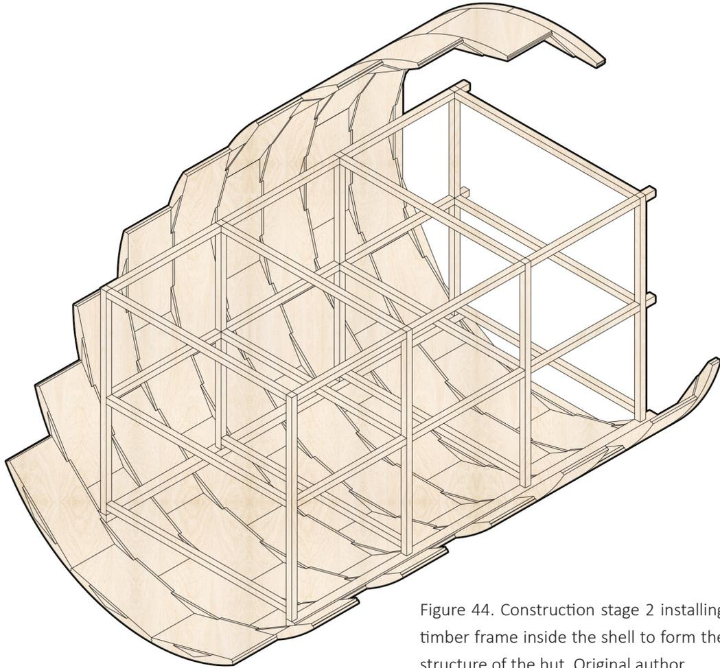
Figure 44. Construction stage 2 installing timber frame inside the shell to form the structure of the hut. Original author
