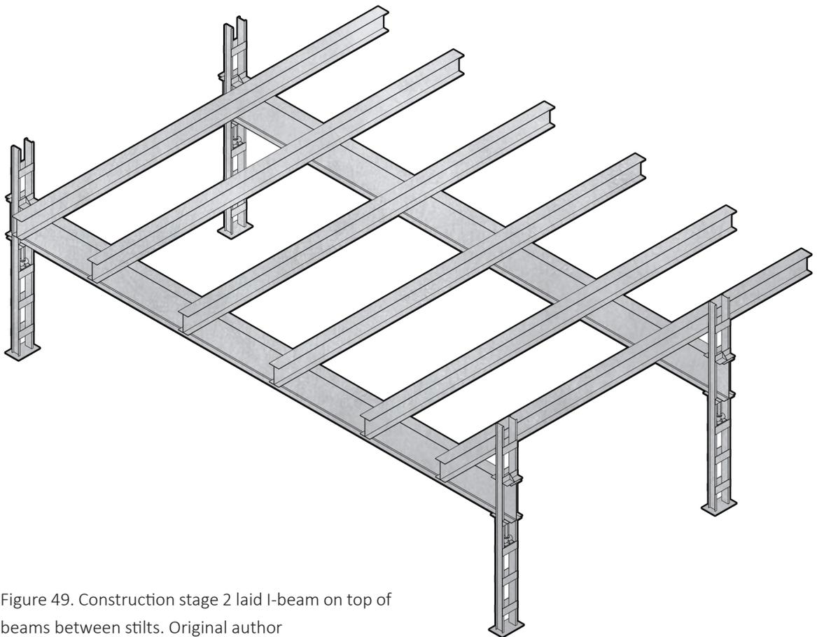
Figure 49. Construction stage 2 laid I-beam on top of beams between stilts. Original author
