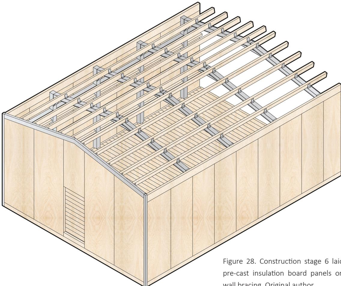
Figure 28. Construction stage 6 laid pre-cast insulation board panels on wall bracing. Original author
