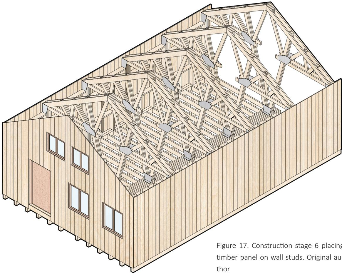
Figure 17. Construction stage 6 placing timber panel on wall studs. Original author
