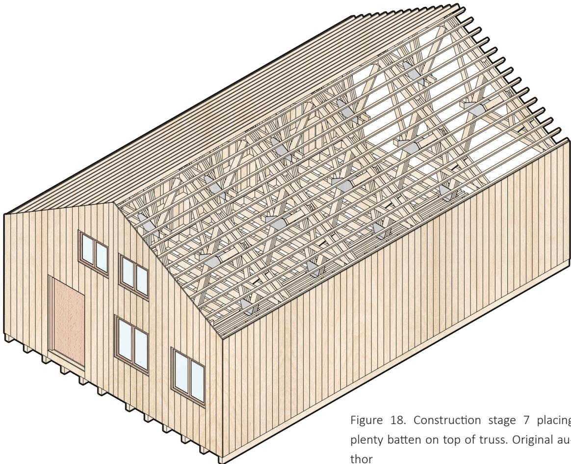
Figure 18. Construction stage 7 placing plenty batten on top of truss. Original author
