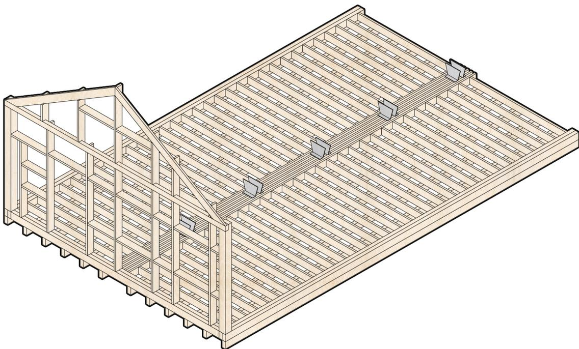
Figure 12. Construction stage 3 placing the frame of entrance to the position. Original author
