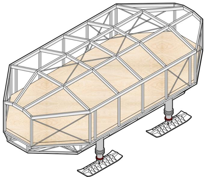
Figure 69. Module of structure construction- stage 4 steel Superstructure was installed on bottom frame. Original author
