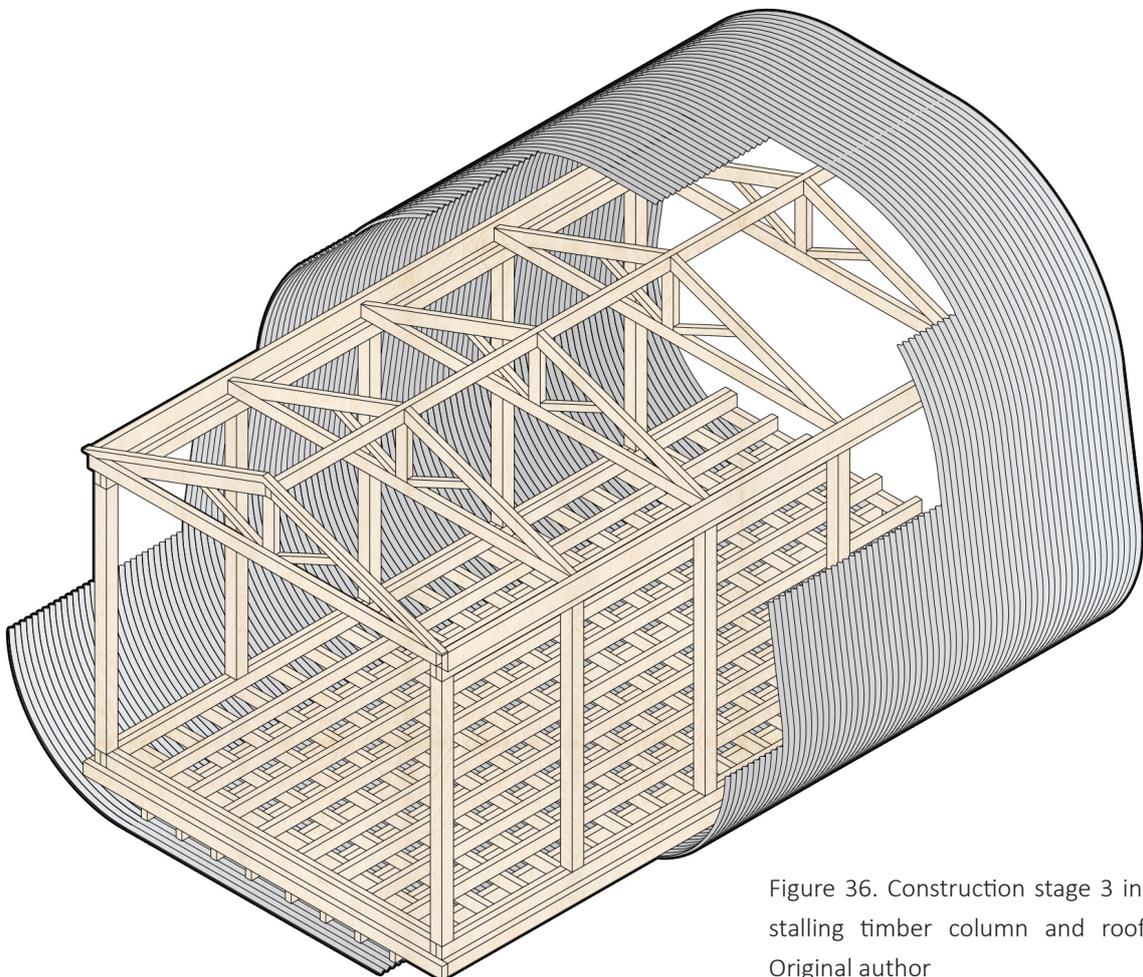
Figure 36. Construction stage 3 installing timber column and roof. Original author
