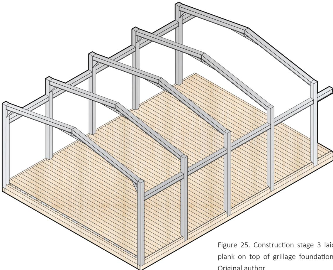
Figure 25. Construction stage 3 laid plank on top of grillage foundation.
