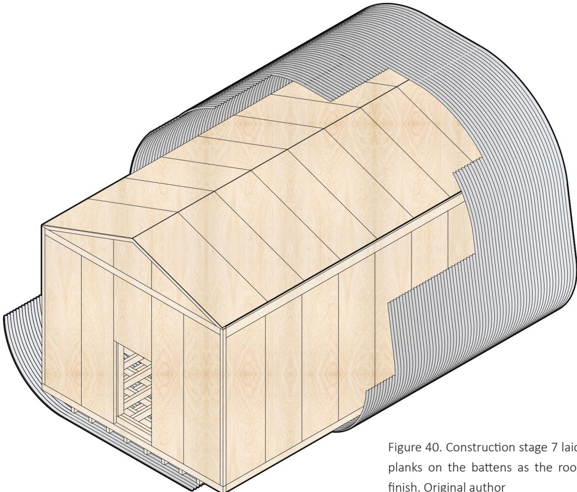
Figure 40. Construction stage 7 laid planks on the battens as the roof finish. Original author
