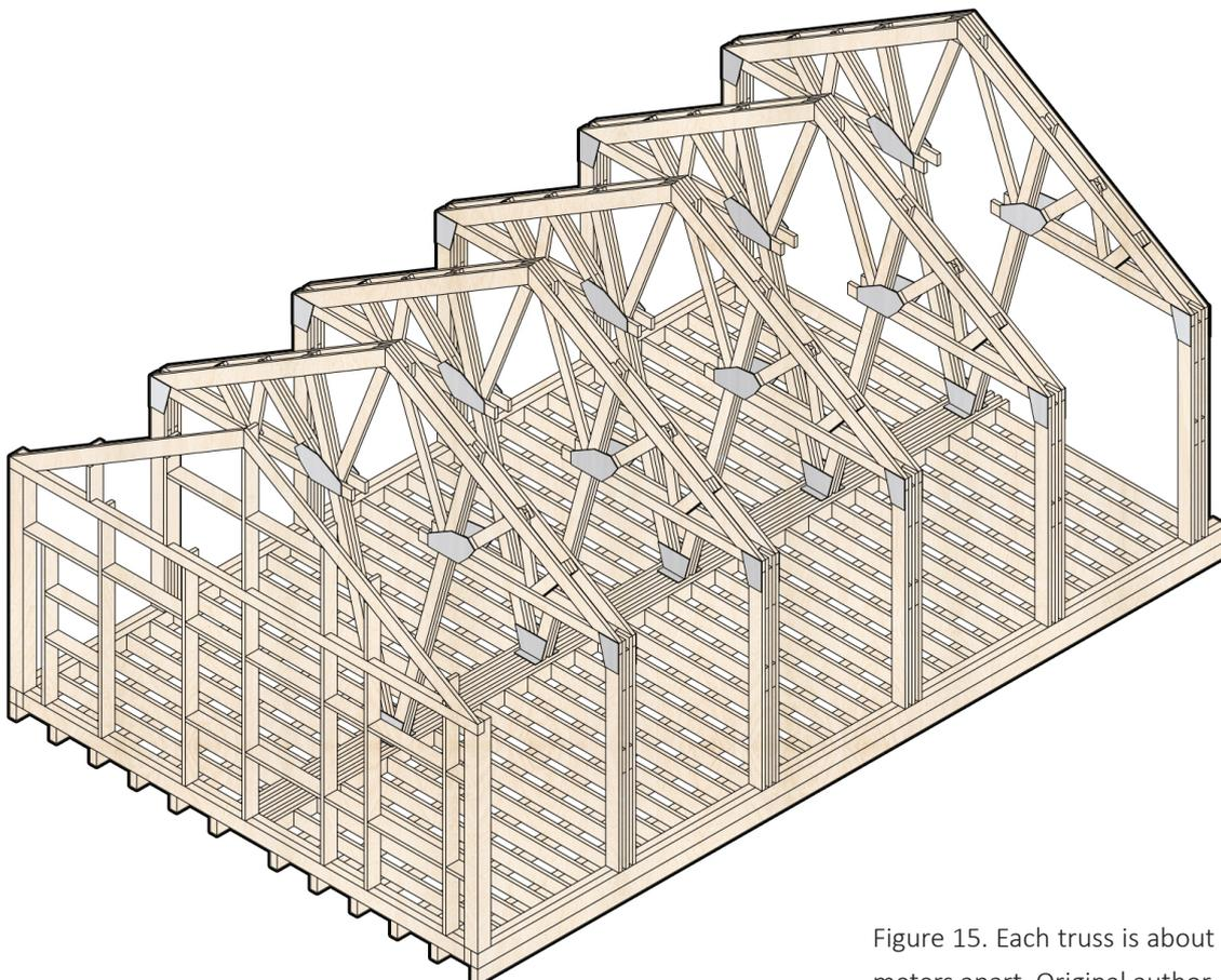
Figure 15. Each truss is about 2 meters apart. Original author
