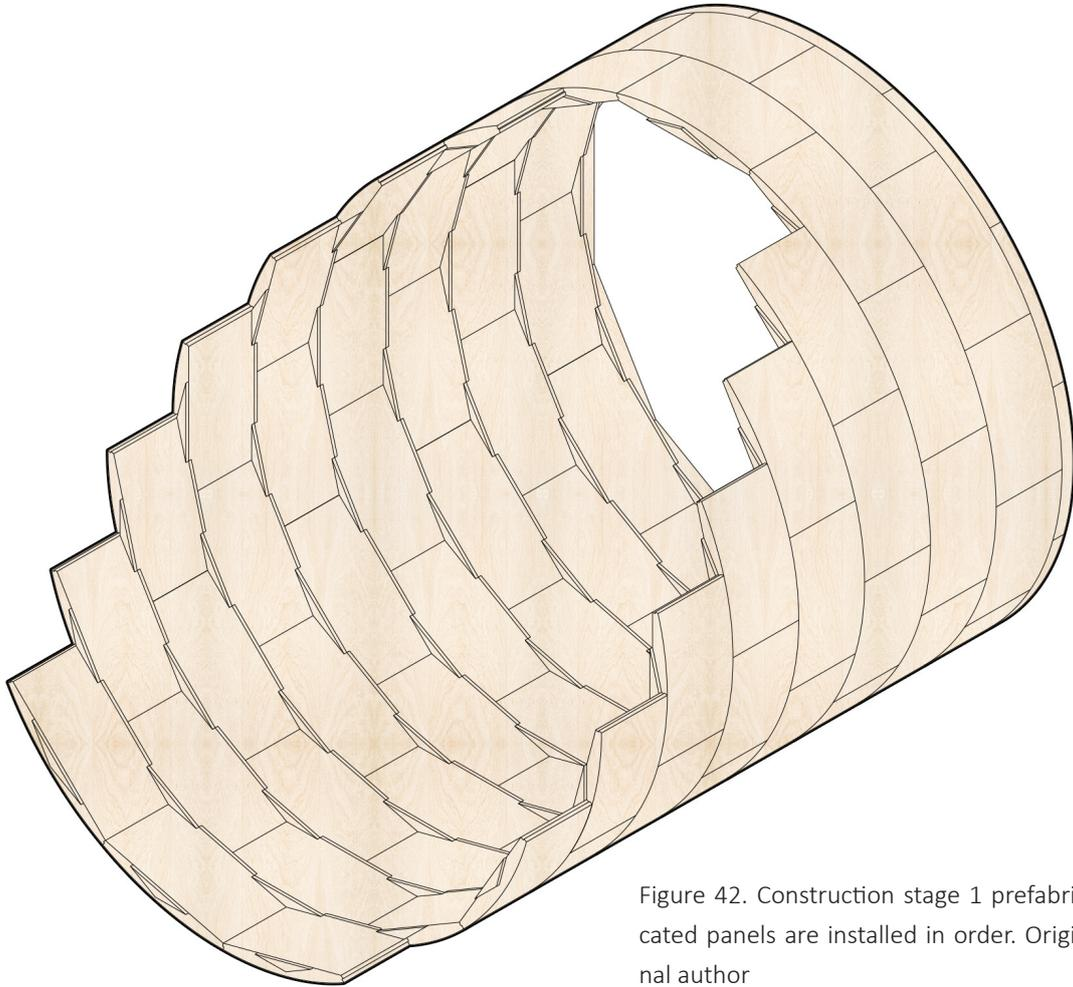
Figure 42. Construction stage 1 prefabricated panels are installed in order. Original author
