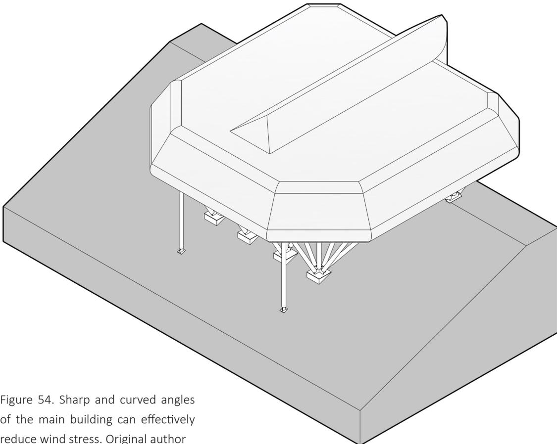
Figure 54. Sharp and curved angles of the main building can effectively reduce wind stress. Original author
