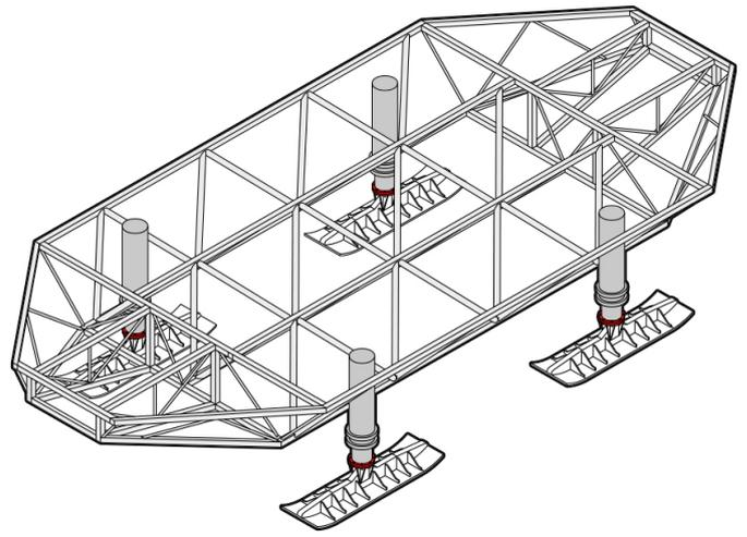
Figure 67. Module of structure construction- stage 2 Hydraulic legs and skis installed. Original author
