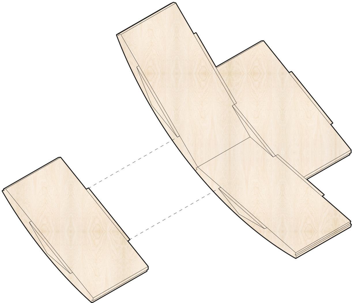
Figure 41. Each prefabricated panel can be interlocked together. Original author
