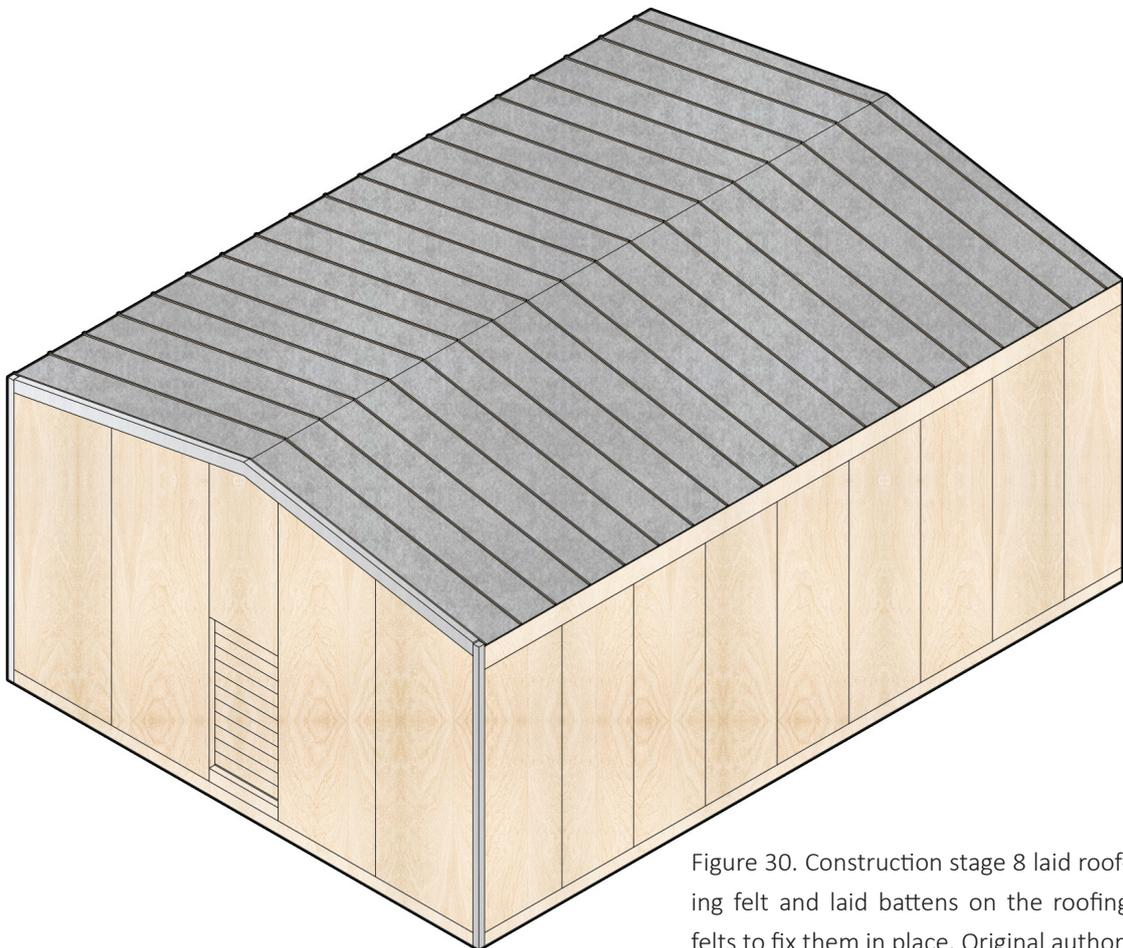
Figure 30. Construction stage 8 laid roofing felt and laid battens on the roofing felts to fix them in place. Original author
