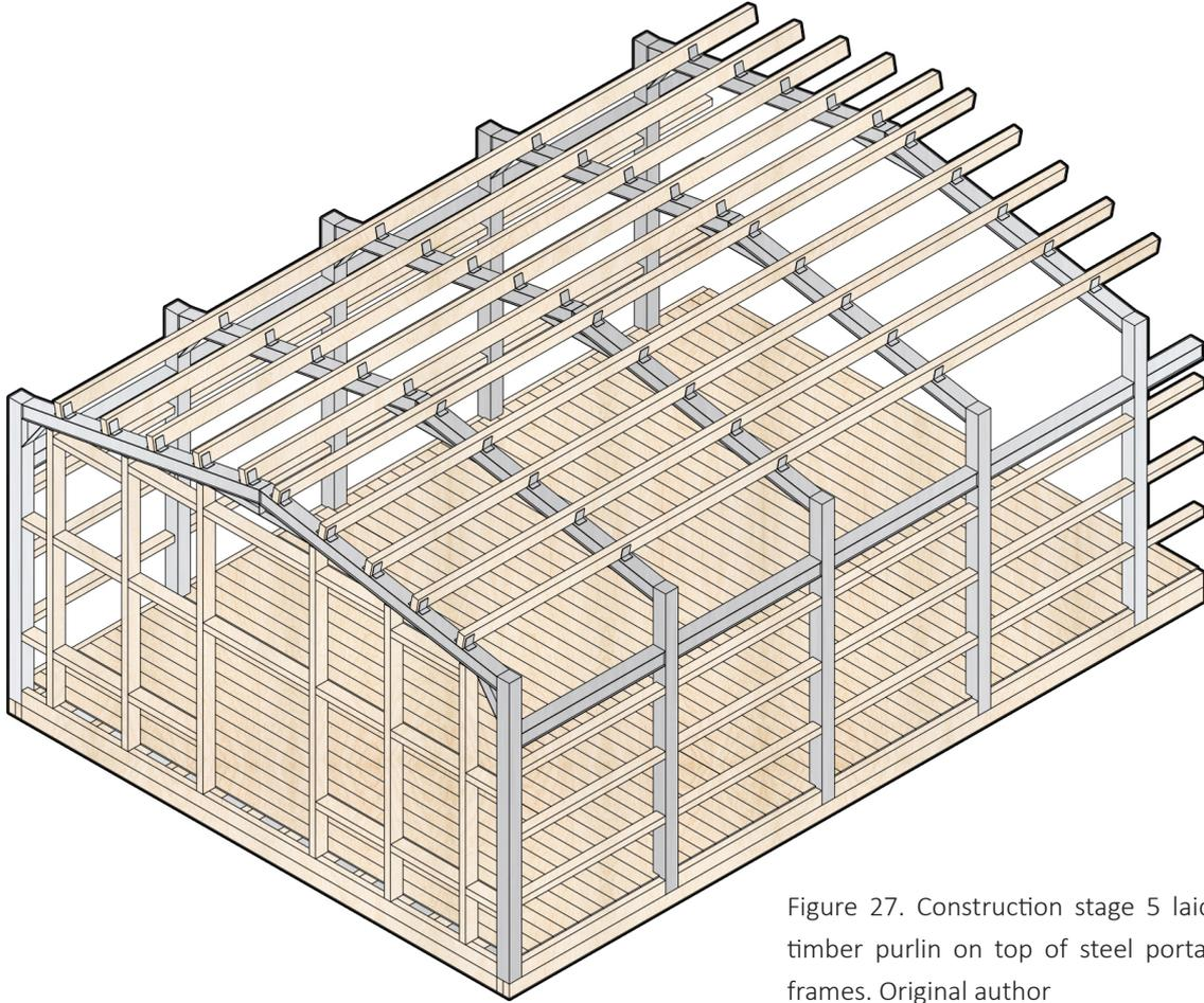
Figure 27. Construction stage 5 laid timber purlin on top of steel portal frames. Original author
