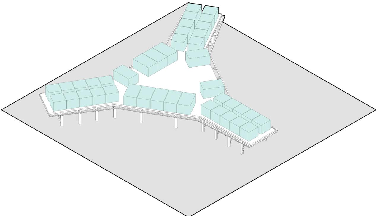
Figure 79. These modules are pre-manufactured in Korea and placed on the platform before the roof structure is installed. Original author
