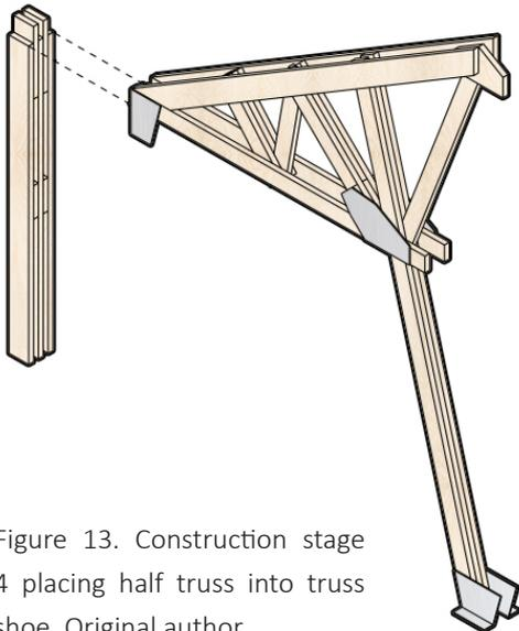
Figure 13. Construction stage 4 placing half truss into truss shoe. Original author
