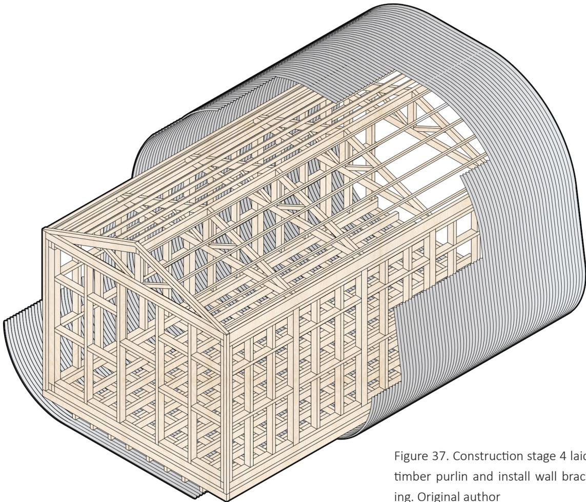
Figure 37. Construction stage 4 laid timber purlin and install wall bracing. Original author
