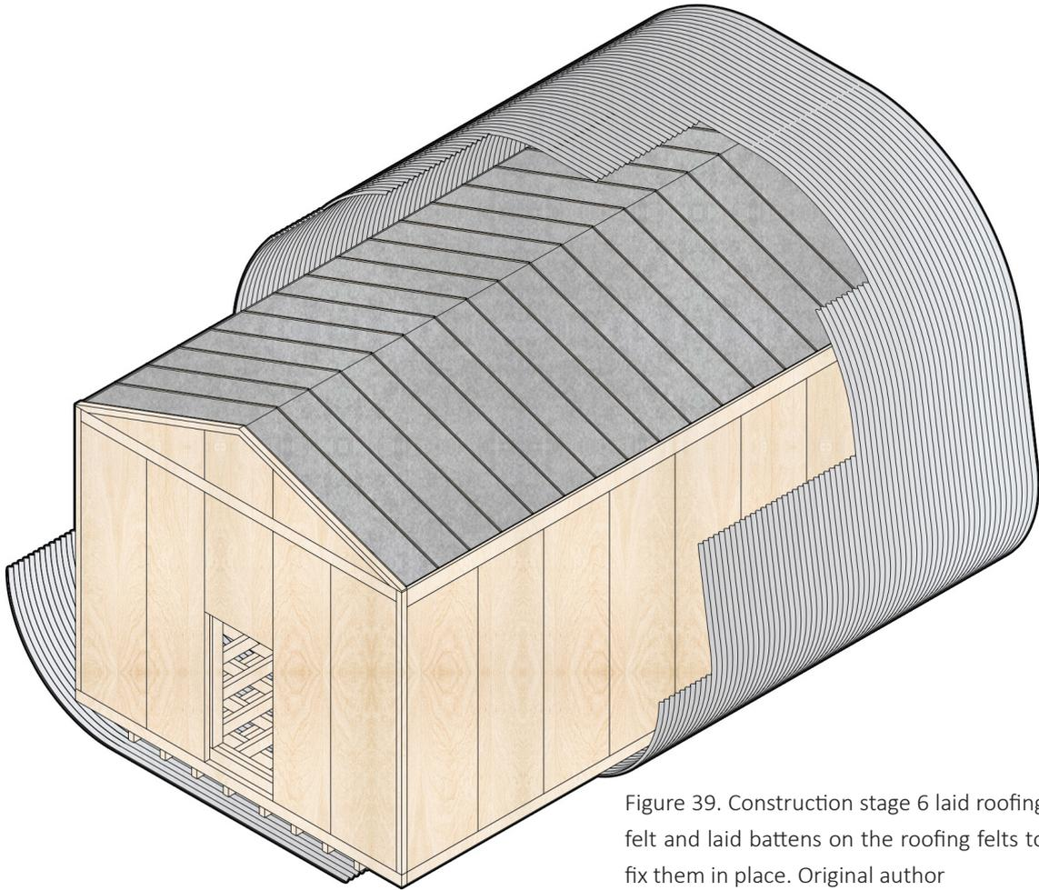
Figure 39. Construction stage 6 laid roofing felt and laid battens on the roofing felts to fix them in place. Original author
