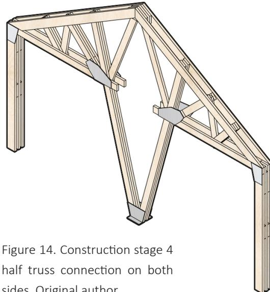
Figure 14. Construction stage 4 half truss connection on both sides. Original author
