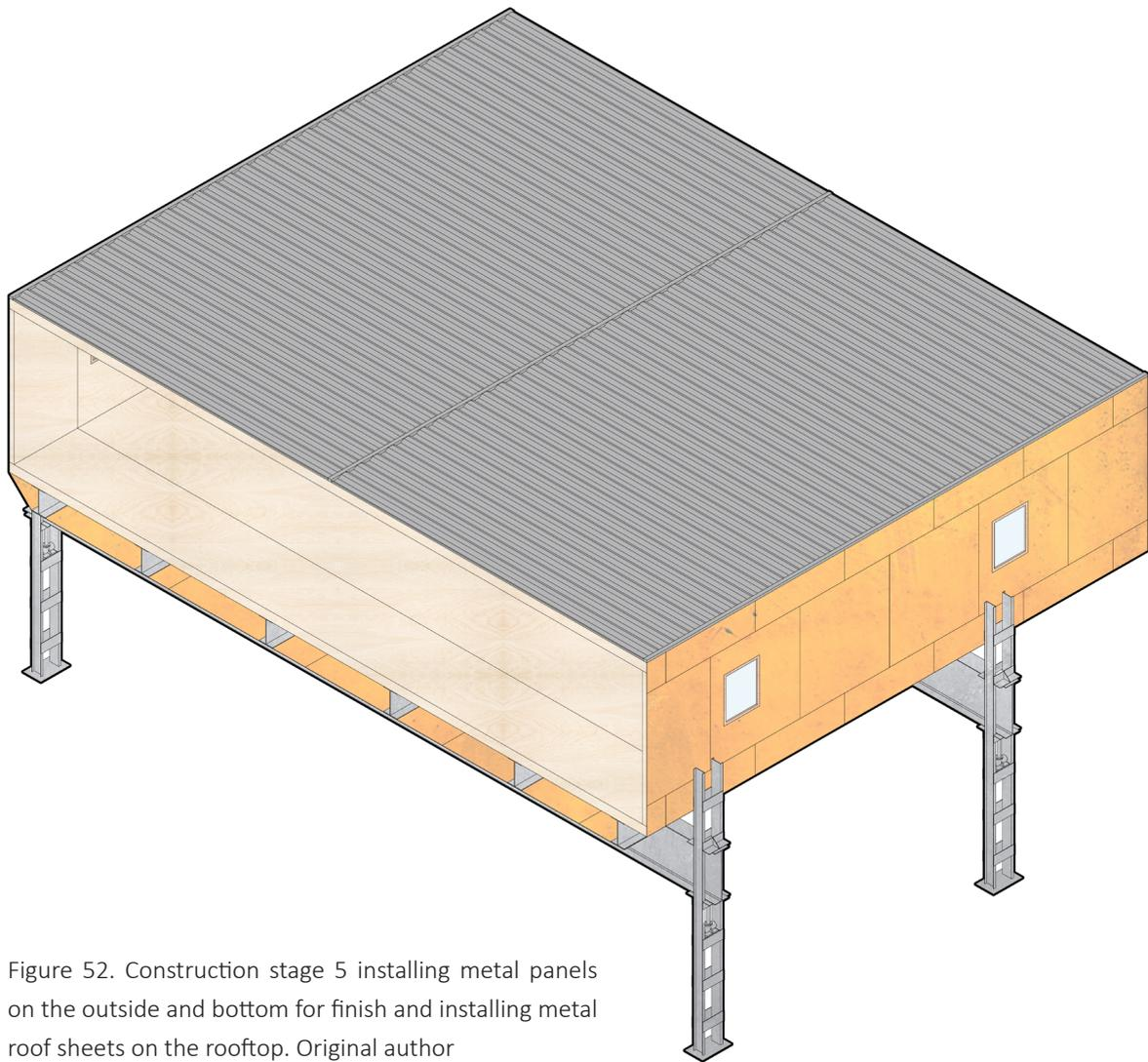
Figure 52. Construction stage 5 installing metal panels on the outside and bottom for finish and installing metal roof sheets on the rooftop. Original author
