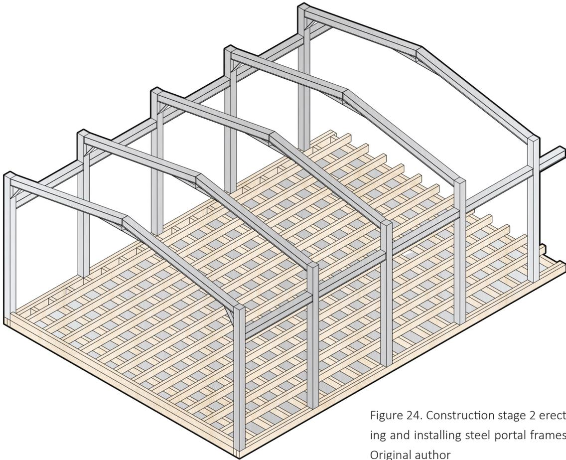
Figure 24. Construction stage 2 erecting and installing steel portal frames.
