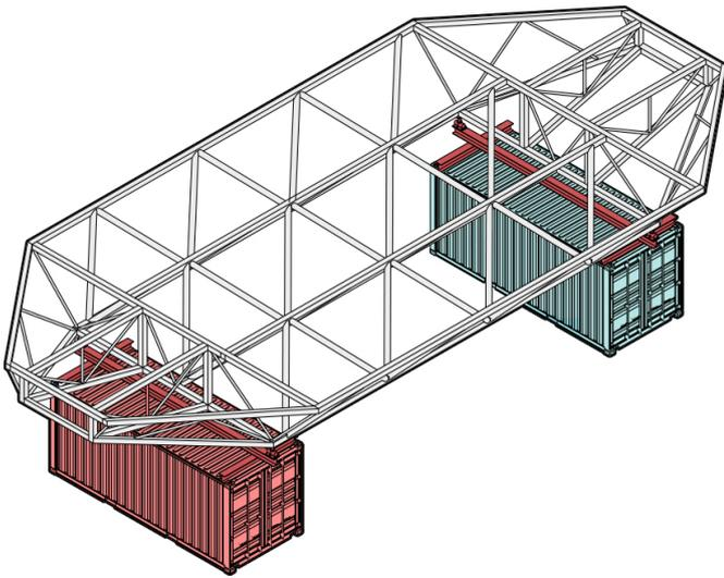
Figure 66. Module of structure construction- stage 1 The module raised on containers to allow hydraulic legs and skis to be installed. Original author
