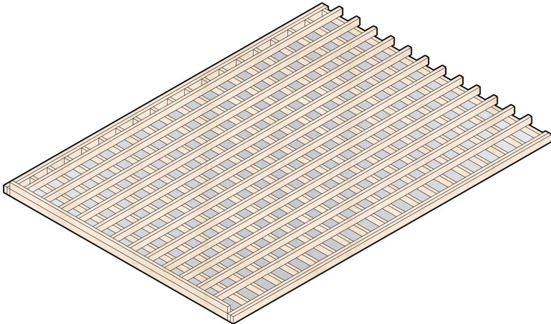
Figure 23. Construction stage 1 placing perforated metal sheet on surface and laid massive of timber on top of metal sheet to form foundation. Original author
