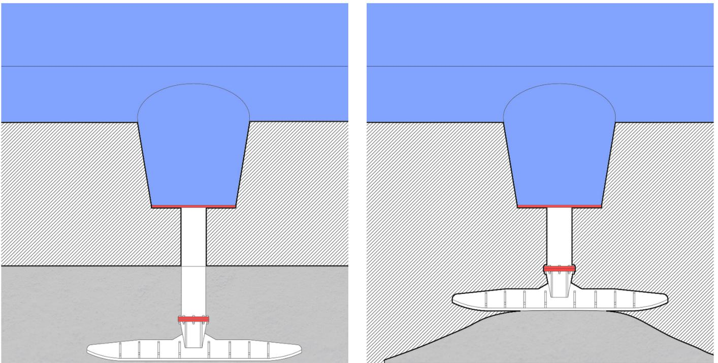
Figure 65. Hydraulically powered legs can be lifted from accumulated snow every year. Original author
